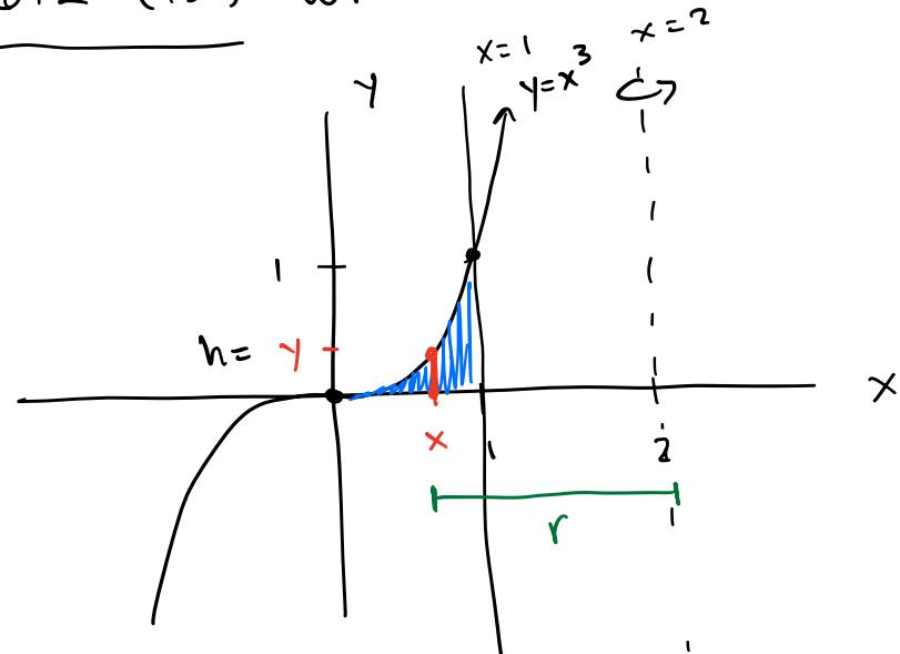
At  $0 \leq x \leq 1$ , we have a thin cylindrical shell of radius  $r = 2 - x$  and height  $h = y = x^3$ .
